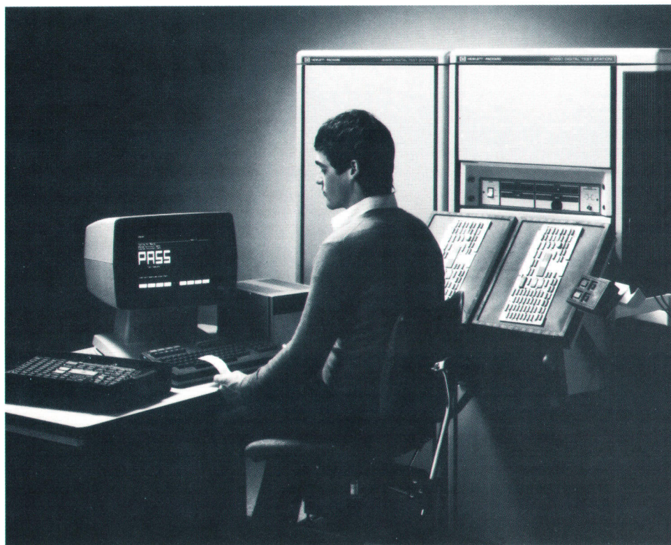
Fig. 1. The HP 3065 Board Test Family provides printed circuit board manufacturers with a combination of high throughput, excellent test quality, and low programming costs for evaluating complex digital and analog circuit boards. The basic configuration shown consists of a measurement section (right), an instrument section (center), and a programming station (left).
